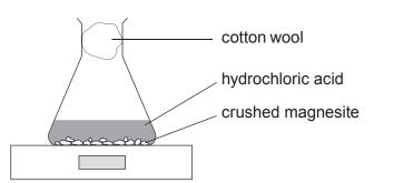
Carbon dioxide was given off during the reaction and the loss in mass was recorded at set intervals.
